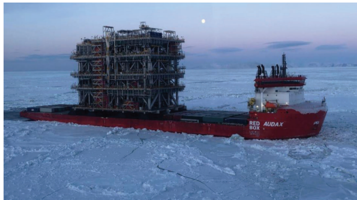
Arc7 ice-class module carrier AUDAX delivers process module for Arctic LNG from Tianjin to Murmansk
