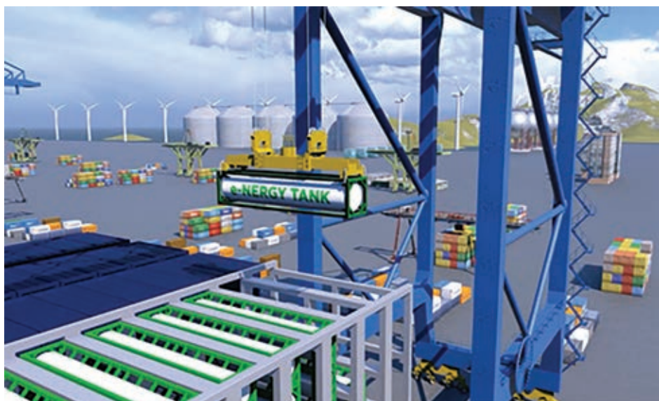
An artist's impression of a tank container being lifted into a deck cell guide structure on board ship
