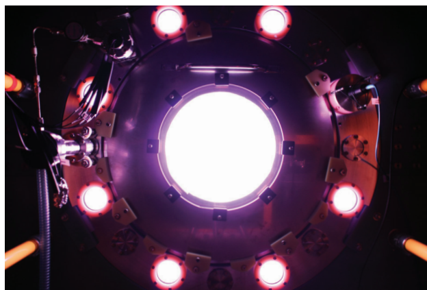
Divertor of Trenta, Helion's 6th fusion generator prototype
