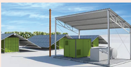
Render of hybrid solar and battery system
