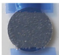
Image of an LTO anode during charging of a typical battery
