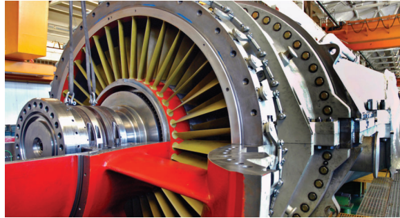
AE64.3A turbine at the factory
