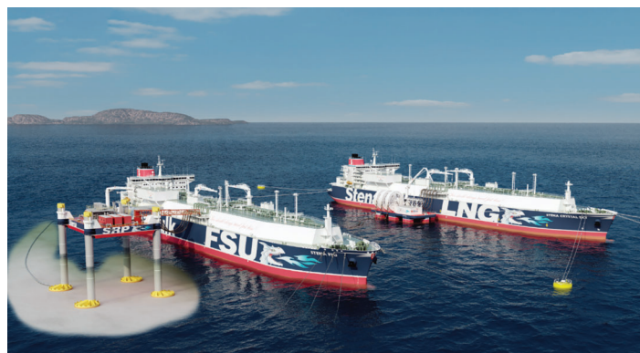
Stena's Jetty-less Floating Terminal and Self-Installing Regas Platform to assist in providing gas-fired power
