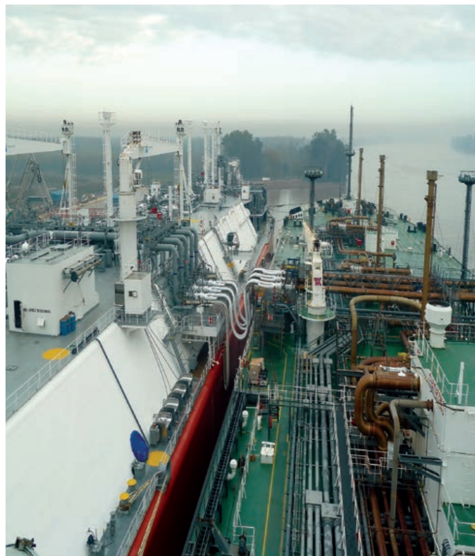
Trelleborg Industrial Solutions' suite of products - SSL Link, QRH, hose breakaway and Gutteling hoses in use in a single LNGC application
