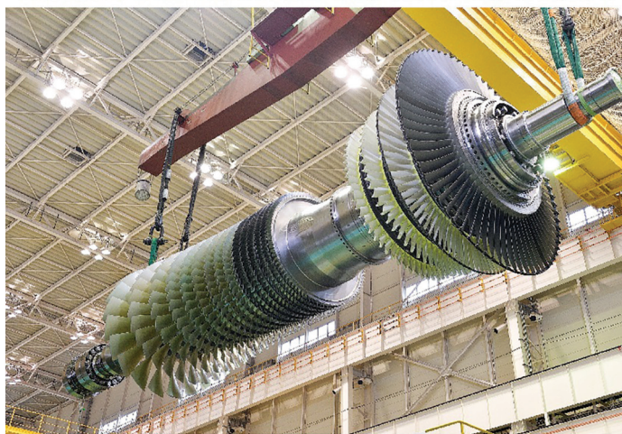
Mitsubishi Hitachi Power System's H501JAC gas turbine
