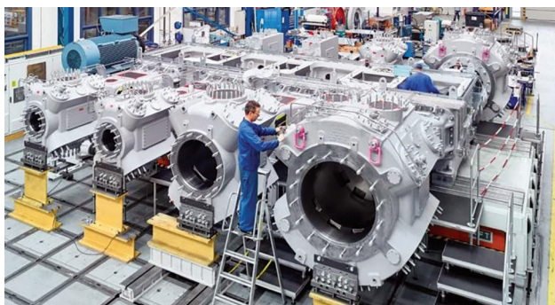
Fine-tuning of a compression unit after manufacturing
