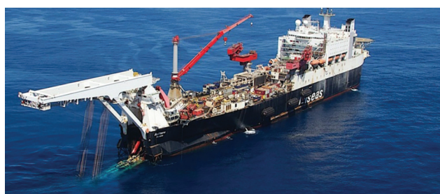
Allseas pipe laying vessel
