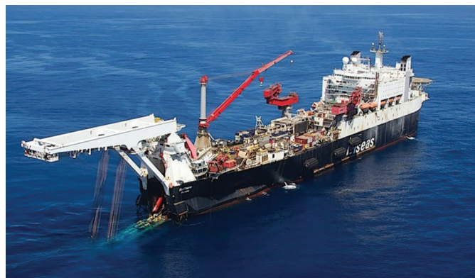
AllSeas' deep sea pipe laying ship Solitaire has been laying most of Nord Stream-2.
