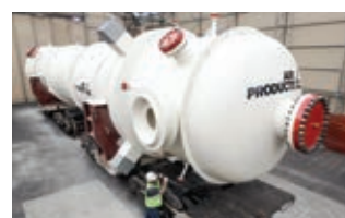
Coil Wound Heat Exchanger
