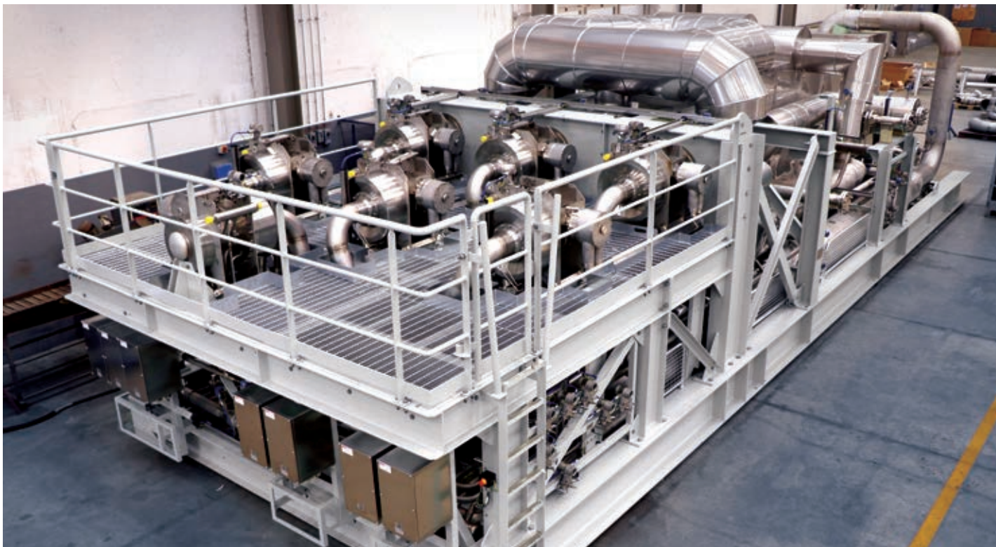
Air Liquide's Turbo-Brayton unit is claimed to be easy to fit on board a gas carrier as it is mounted on a skid
