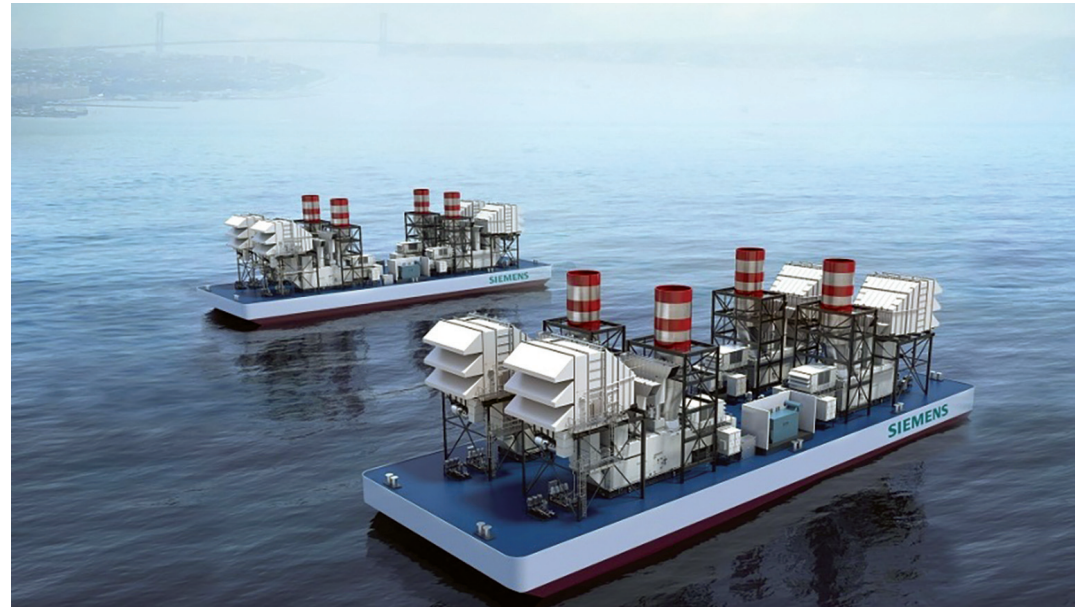
SeaFloat power barges with four SGT-A65 gas turbines
