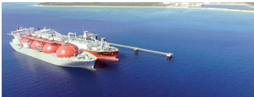
The FSRU 'Exemplar' and the LNGC 'Arctic Voyager' seen conducting the Bahamas LNG transfer operation
