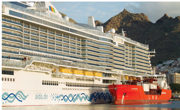
The converted small-scale LNGC 'Coral Methane' recently bunker the LNG powered 'AIDAnova' at Tenerife.
