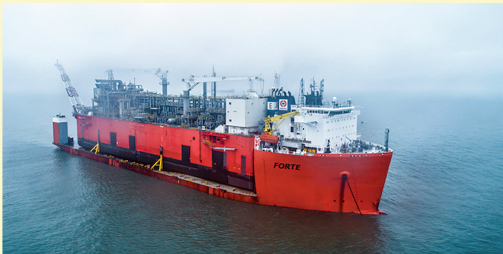
'Tango FLNG' is being transported to Argentina on board a semi-submersible heavy lift ship
