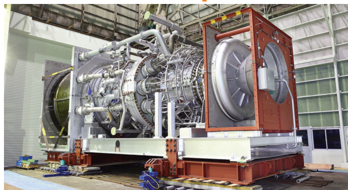
The H-100 gas turbine and compressor package ordered for Africa for Exxon Mobil-run export joint venture
