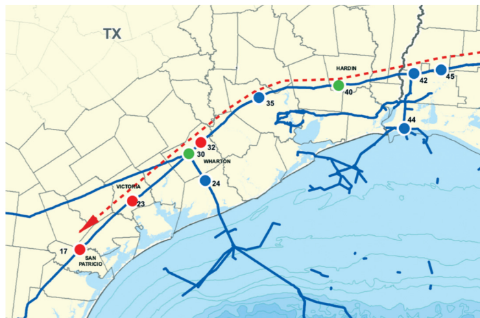
Gulf pipeline includes reverse flow at station 40 and new compressors at stations numbered 17, 23 and 32
