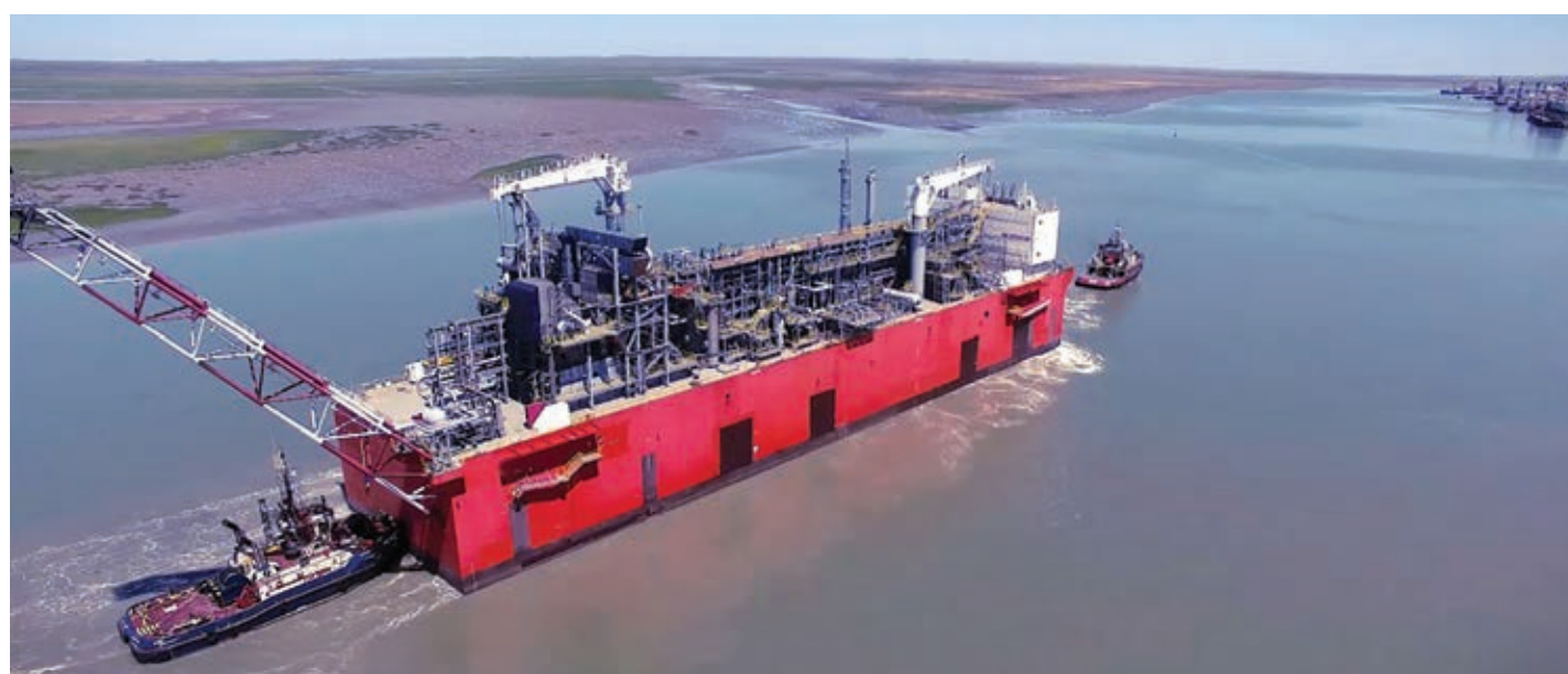
Exmar's 'Tango FLNG' arrives at Bahia Blanca port in Argentina. The Black & Veatch liquefaction process was installed during construction and when it was originally bound for off the Caribbean coast of Colombia
