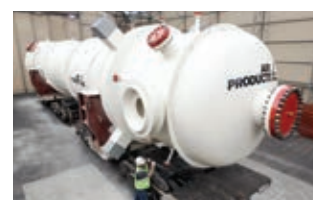
Coil Wound Heat Exchanger
