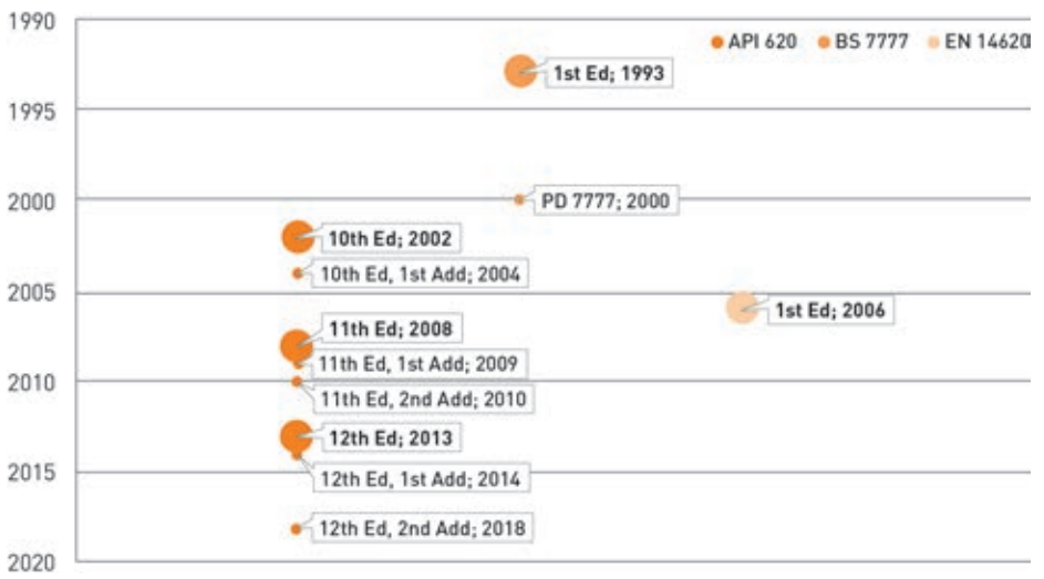
Figure 1: Revision history of selected LNG tank codes
