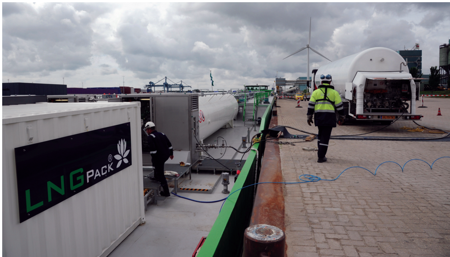
LNG refuelling operation at Rotterdam
