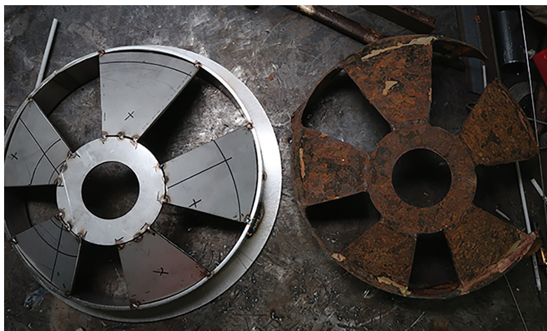
Corrosion on scrubber diffuser
