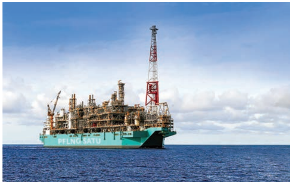
The ‘PFLNG Satu’ hull owned by Malaysia’s Petronas was a world first. It produces LNG from the Kanowit natural gas field offshore Sarawak
