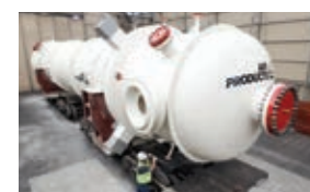
Coil Wound Heat Exchanger
