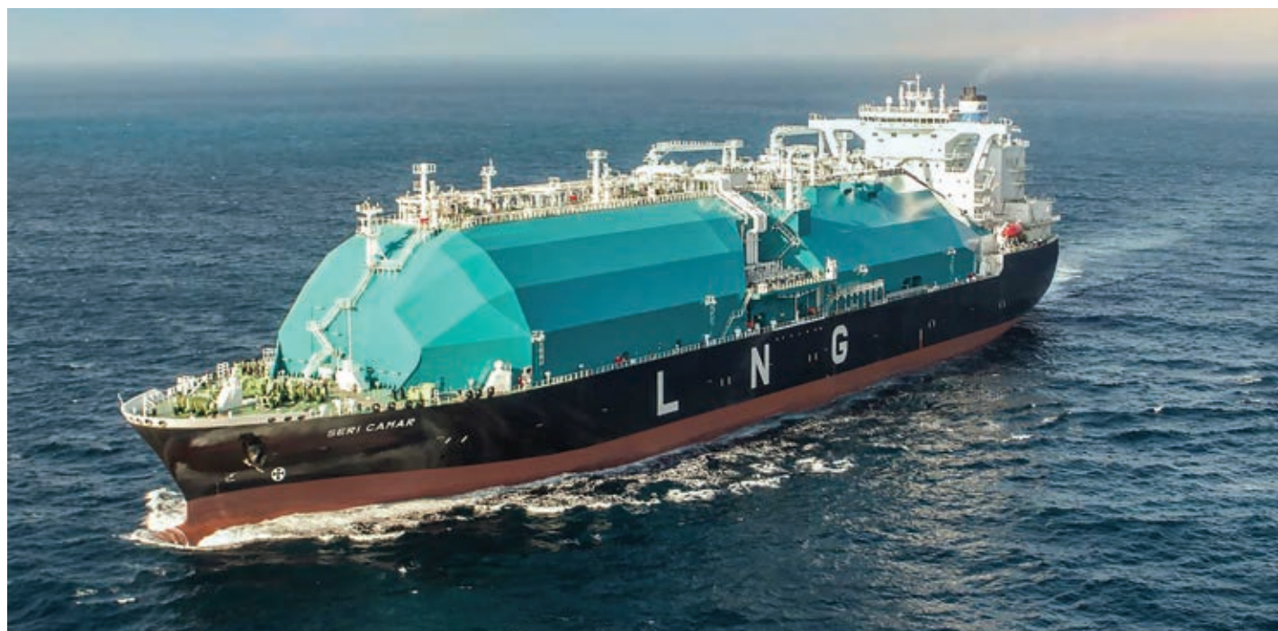
The 150,200 cubic metres capacity carrier ‘Seri Camar’ was built at Hyundai and has covered Moss tanks
