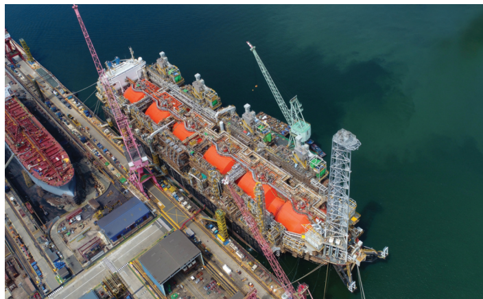
The world's first FLNGV conversion is nearing completion in Singapore
