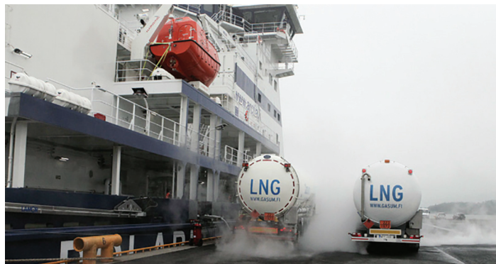
Ships can take on LNG from trucks or other vessels
