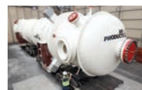
Coil Wound Heat Exchanger
