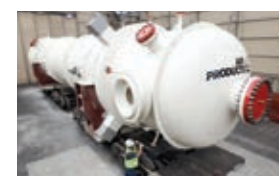
Coil Wound Heat Exchanger
