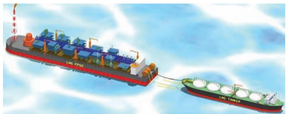
Offshore LNG production and transfer concept ( https://www.chiyoda-corp.com/technology/en/lng/offshore.html )
