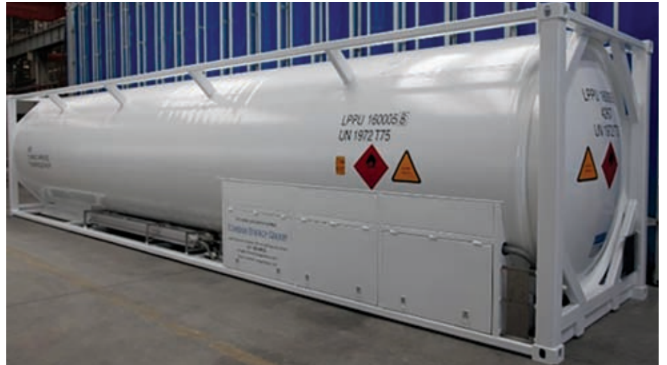
One of 12 ISO LNG tank containers supplied to coal-fired plant
