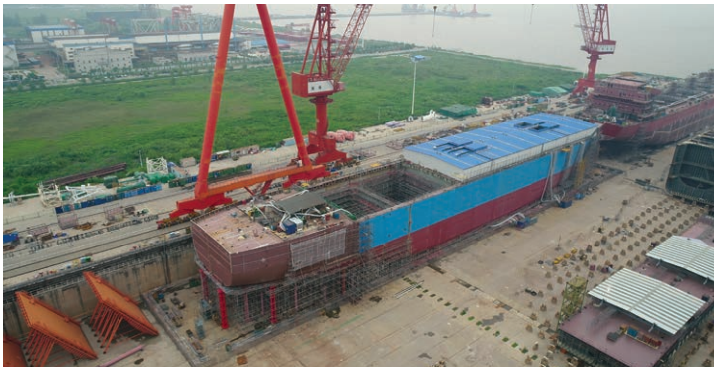
Hull of the LNT45 45,000 cu m LNGC seen under construction at China Merchant's shipyard.
