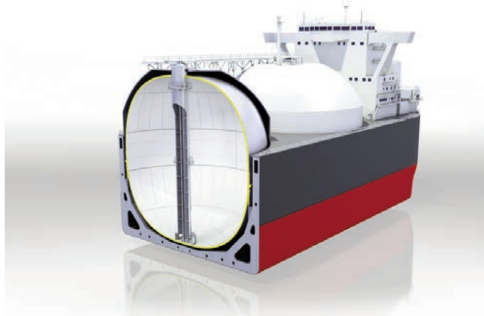
KHI's new non-spherical (MOSS) tank is a IMO Independent Type B LNG tank that has been developed for use in 180,000 cu m LNGCs. Credit: KHI.
