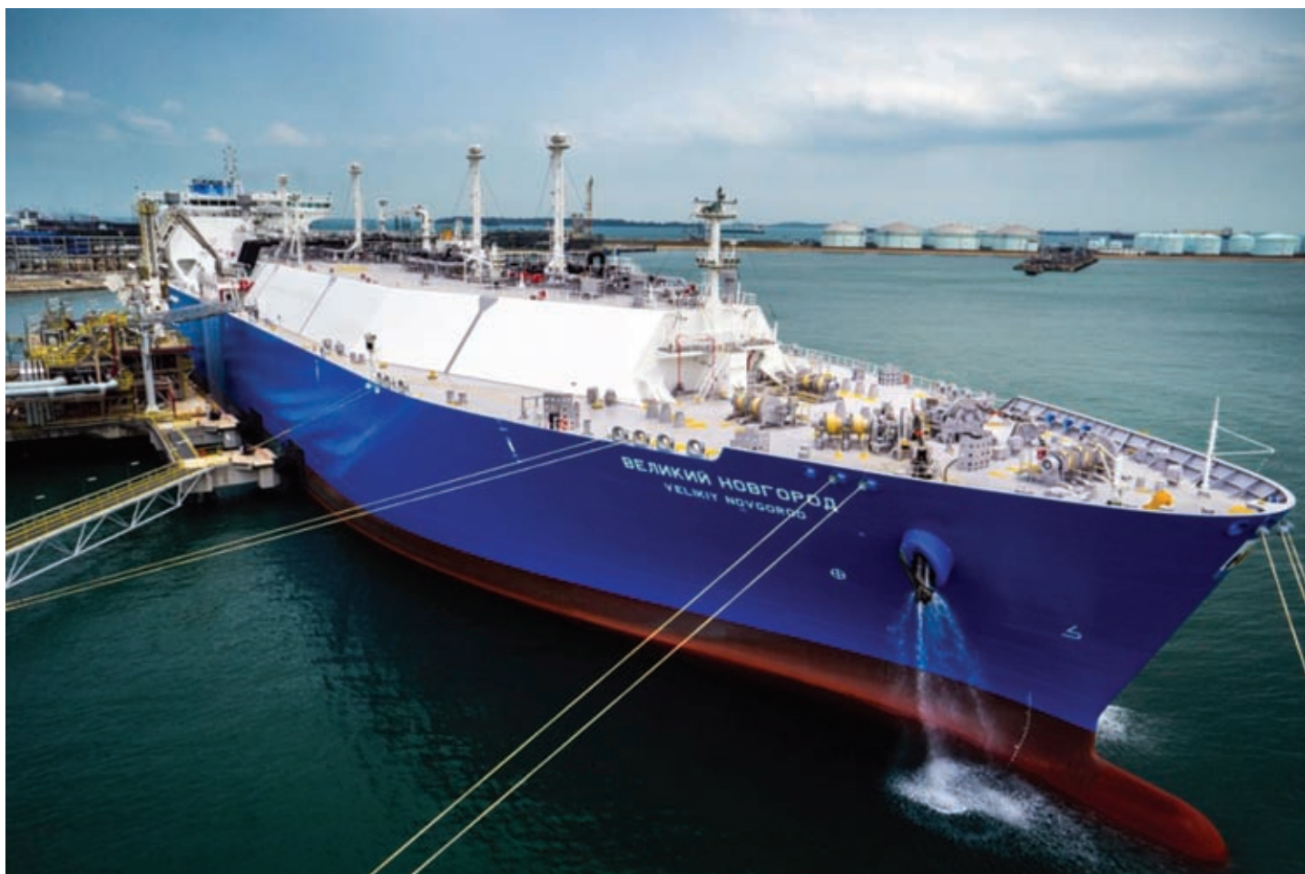
SCF's first 170,000 cu m ice class LNGC Velikiy Novgorod will eventually serve the Yamal project.
