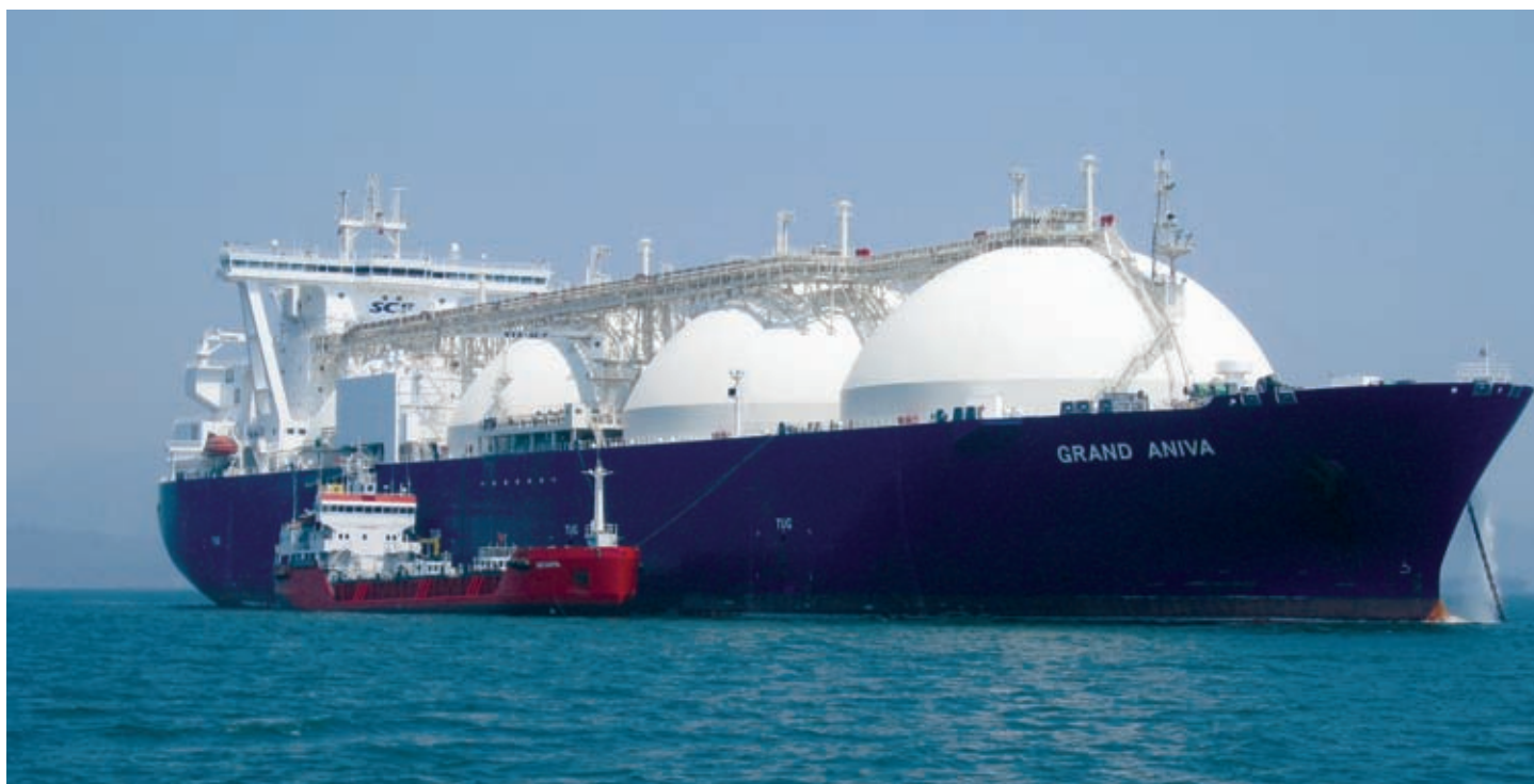
SCF's 145,000 cu m Grand Aniva seen bunkering at Nakhodka. She was the first gas ship to bunker at the Russian Far East port. Note enclosed bridge for harsh weather operations.
