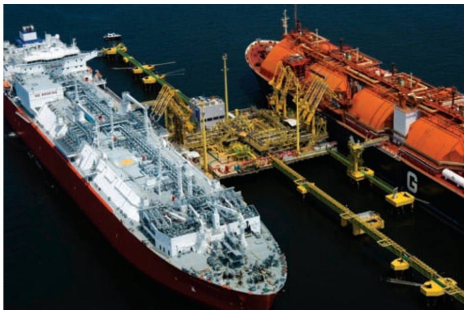
One of Exmar's LNGCs seen adjacent to a Golar FSRU in Brazil, operating for Petrobras.
