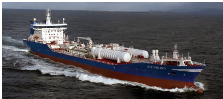
Since her conversion to gas burning, Tarbet Shipping's Bit Viking has operated over 3,000 hours in gas mode.
