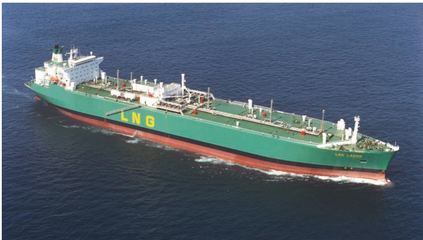
The veteran 122,255 cu m LNG Lagos was built in 1976 and is managed by Shell for the Nigeria LNG operation. She is fitted with a GT No 85 containment system.
