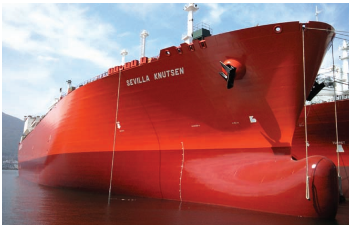
The 173,400 cu m Sevilla Knutsen is currently operating for Stream. She was built in 2010 and is fitted with a GT No 96 containment system.
