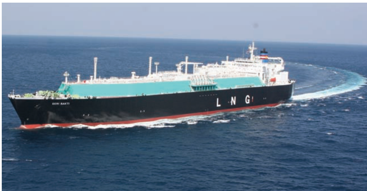
MISC's 152,944 cu m Seri Bakti is fitted with a GT No 96 containment system and was delivered in 2007.
