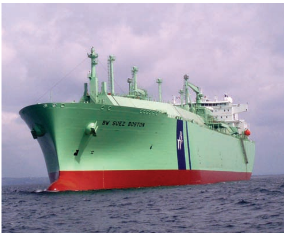
The BW Gas managed 138,059 cu m BW Suez Boston was built in 2003 and fitted with a GT No 96 containment system. She is 51% owned by BW Gas and 49% by Distrigas.
