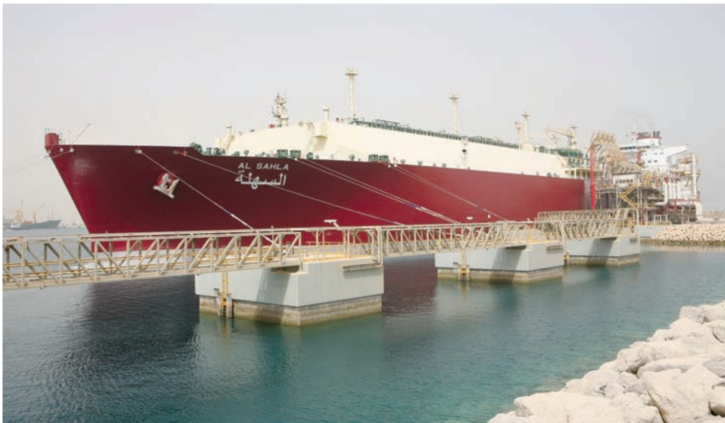
The J5 Nakilat owned, NYK LNG Ship Management managed 216,200 cu m Q-flex Al Sahla was delivered in 2008 and has a Technigaz Mk III containment system fitted.
