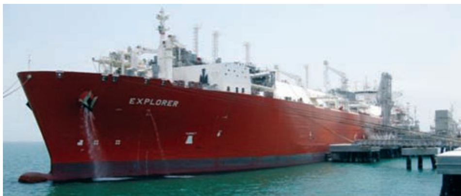
Exmar/Excelerate's 150,981 cu m LNGRV Explorer seen alongside Kuwait's Mena al Ahmadi gas receiving terminal. She is fitted with a GT No 96 containment system and was delivered in 2008.
