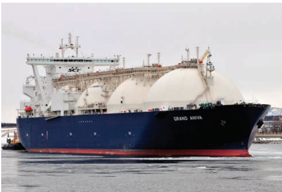
SCF's 145,000 cu m Grand Aniva was delivered in 2008 and as can be seen is fitted with a Moss system.
