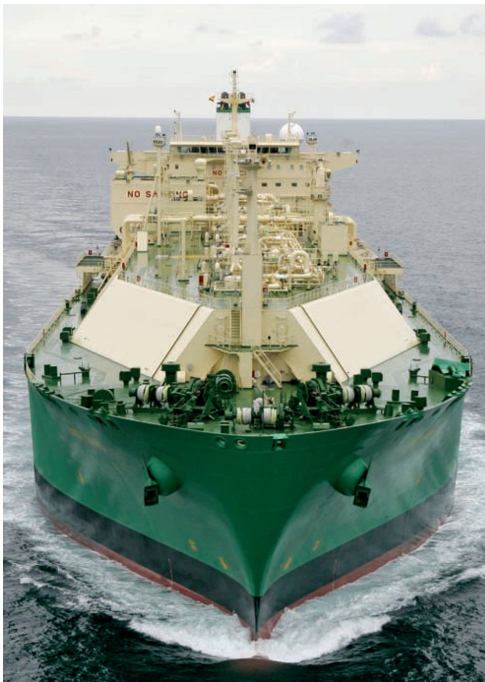
BW Gas also manages the 148,565 cu m LNG Kano. She was built in 2007 and also fitted with a GT No 96 containment system.
