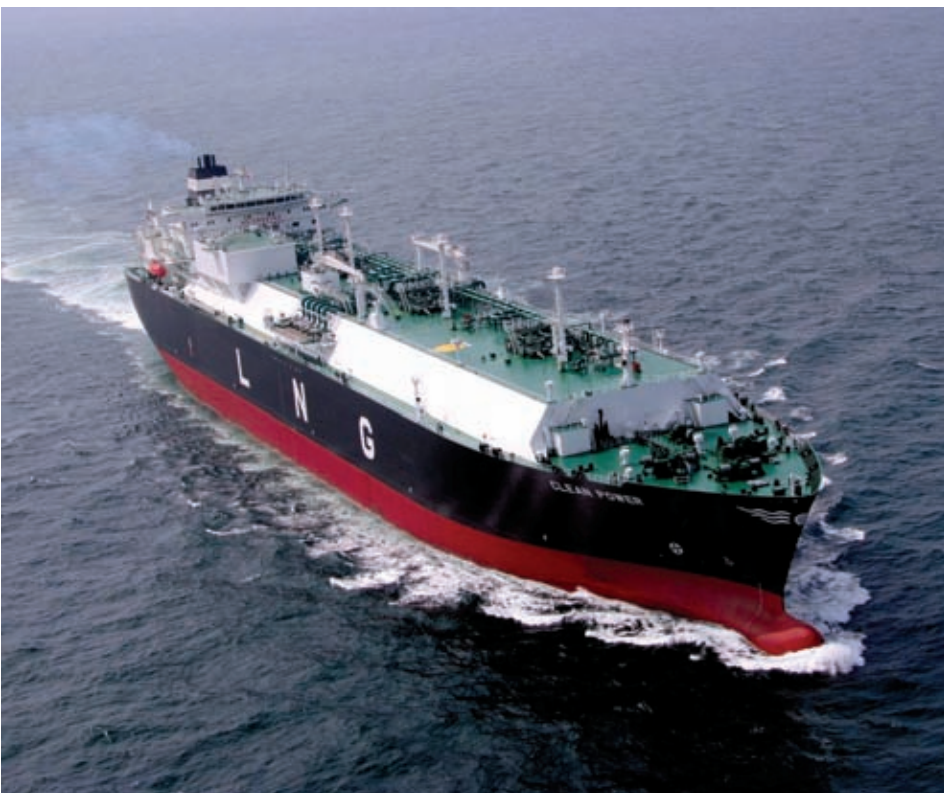
Dynagas' second ice class 149,700 cu m, Technigaz Mk III type LNGC was delivered in 2008.
