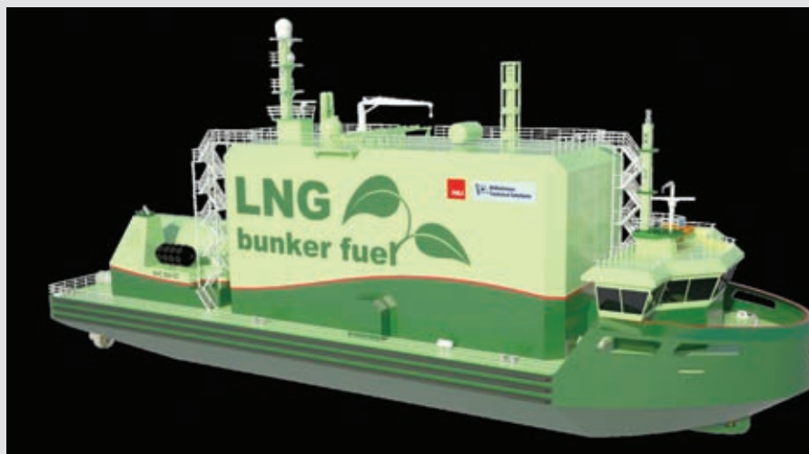
NLI Solutions' LNG bunker barge design.
