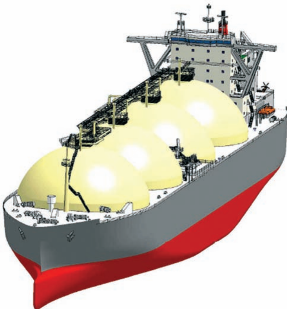
Kawasaki has ordered a Moss type 164,700 cu m LNG from KHI. This vessel will be built to a new hull design aimed at greater cargo carrying capacity.
