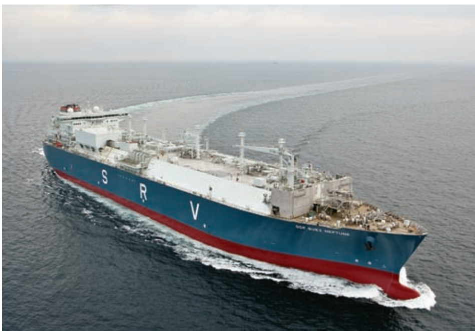
The 2009-built 145,130 cu m GDF Suez Neptune is jointly owned by MOL and Hoegh LNG. She is fitted with a Technigaz Mk III containment system.
