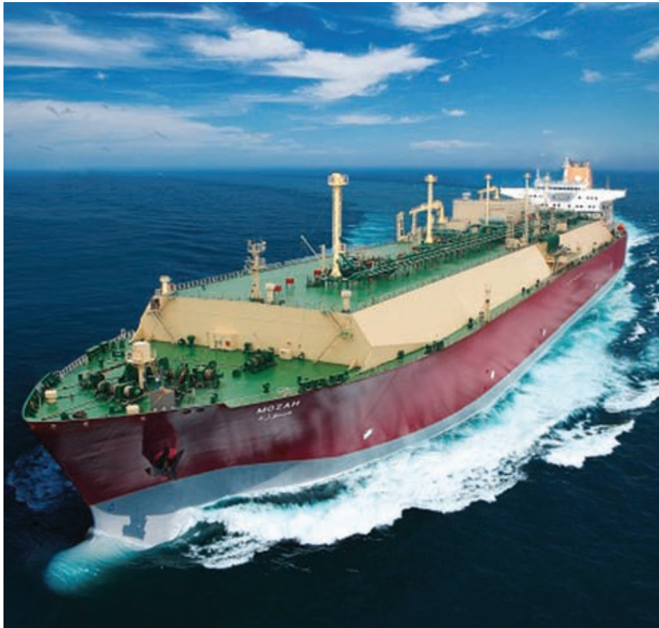
The Shell managed and operated Q-Max Mozah has a capacity of 266,000 cu m, was delivered to Nakilat in 2008 and is fitted with a Technigaz Mk III containment system.
