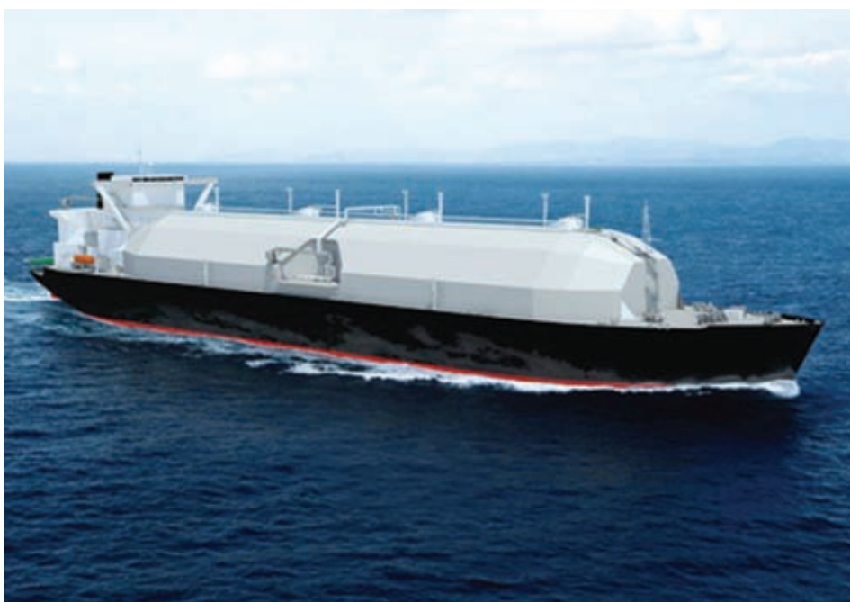
MOL has ordered a 155,300 cu m 'Sayaendo' type LNGC developed by Mitsubishi. This design features a continuous cover over its Moss type tanks.
