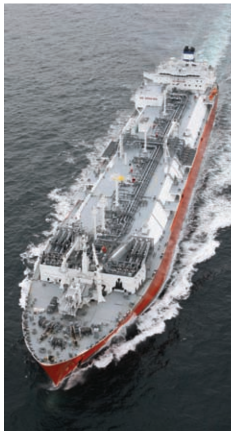
Express - one of Exmar's new generation 151,000 cu m LNGRVs. Photo credit - Exmar.
