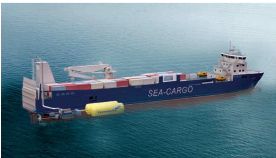
An illustration of a SeaCargo vessel fitted with Hamworthy’s LNG fuel tank.
