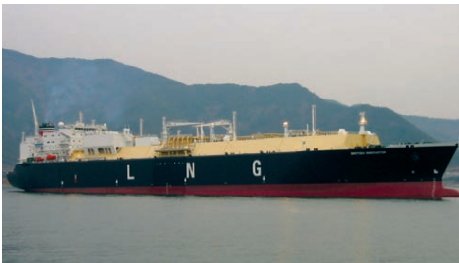
A BP dual fuel diesel-electric LNGC.
