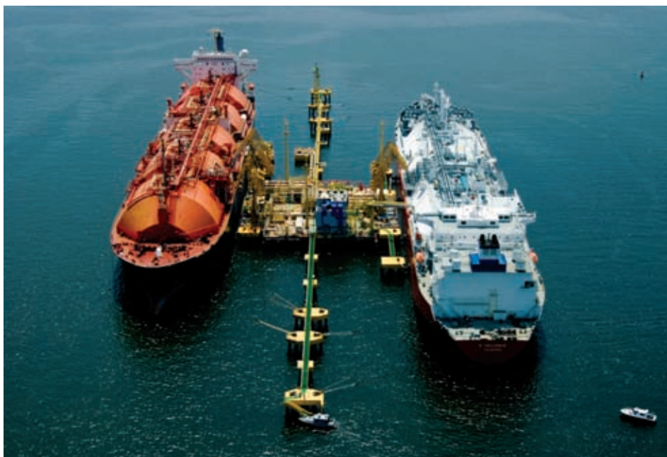
A Moss-type Golar FSRU in operation for Petrobras.
