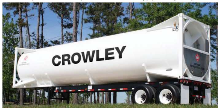
Crowley will use ISO containers to supply LNG to clients in Alaska. (Source: Crowley)
