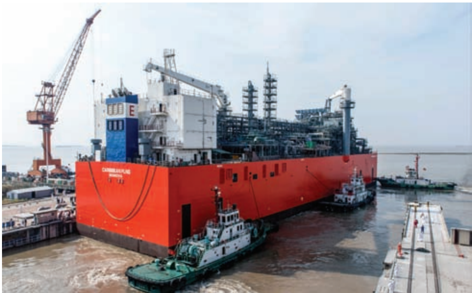
EXMAR’s FLNG hull, a barge for liquefaction and temporary storage
