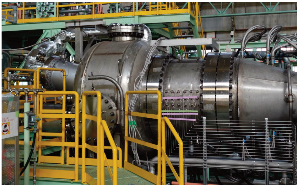
Test stand demonstrating ammonia combustion at GE turbine
