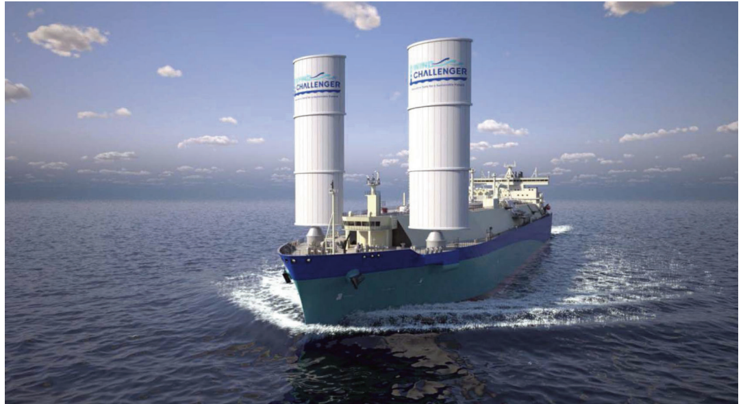
An impression of MOL's LNGC fitted with sails
