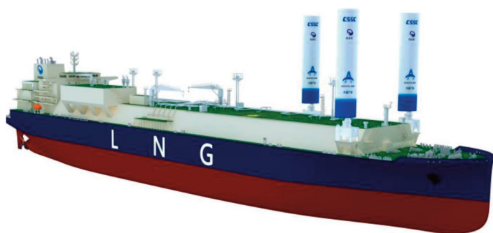
The design concept has the sails located near the bow
