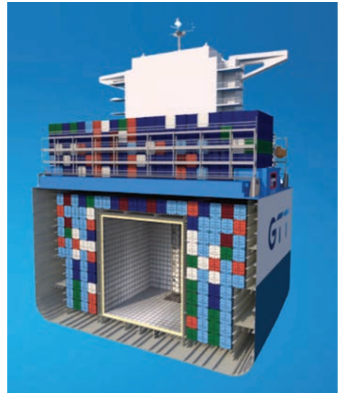
CUBIQ system features chamfer-less design
