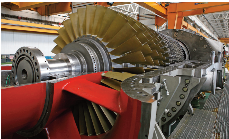
Close-up of AE94.3A gas turbine
