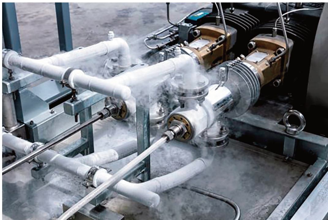
Vanzetti's VT-3 duplex high-pressure reciprocating pumps
