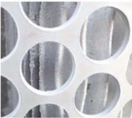
Cargo manifold strainer 60 mesh size – partially clogged. Source: Brookes Bell
