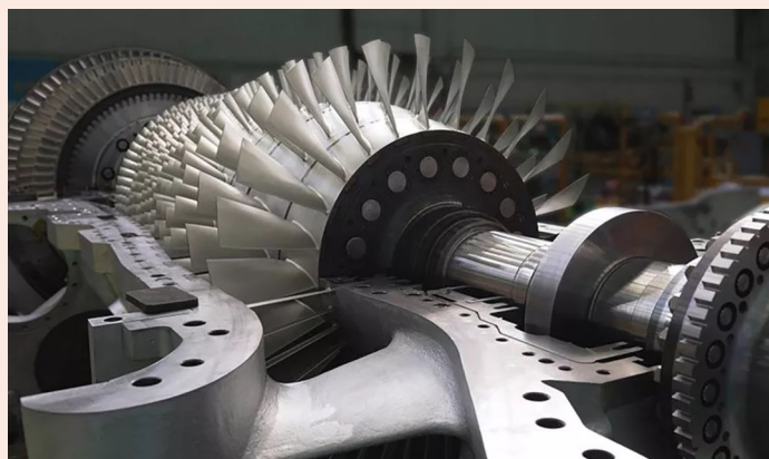
Close-up of H-25 Series gas turbine
