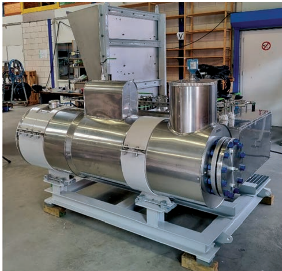
The flow meters are built on skids
