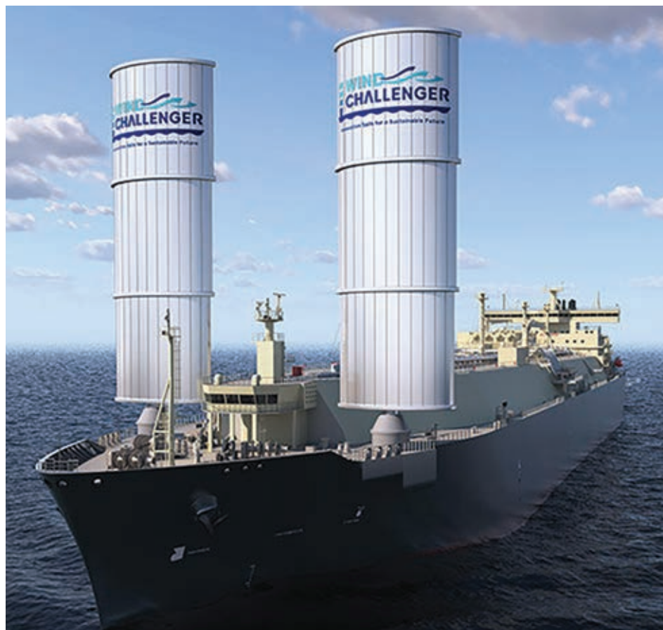
MOL Encean equipped with Wind Challenger system
